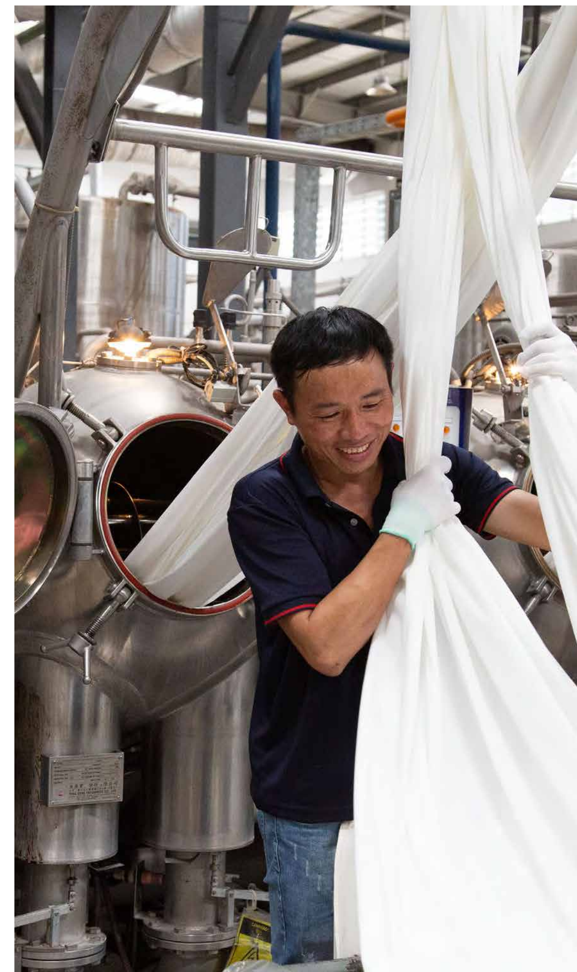
Teammates at a Far Eastern facility in Vietnam load a dye machine with fabric made from recycled polyester.
