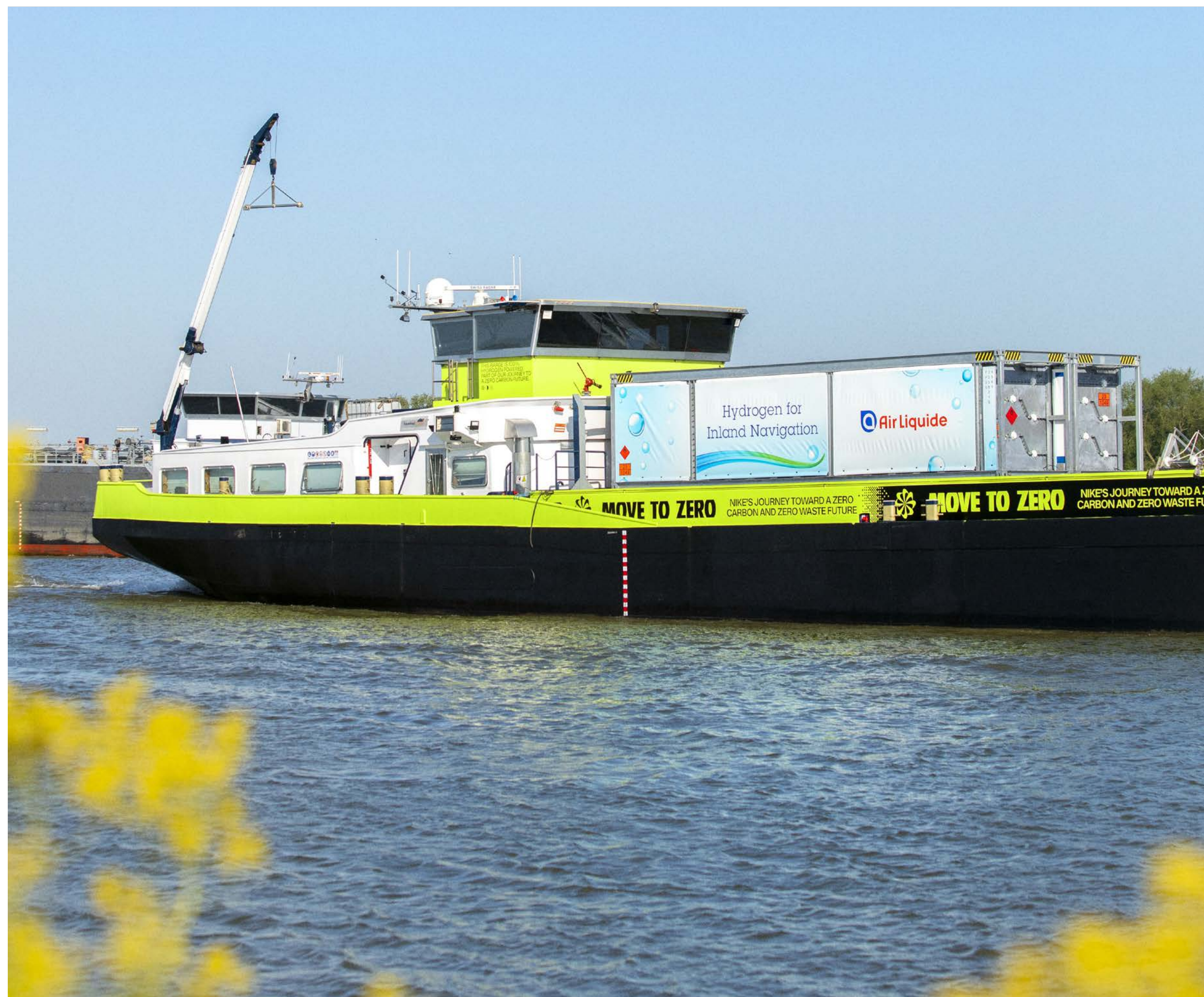
The H 2 Barge 1, a zero-carbon-dioxide-emissions inland vessel
