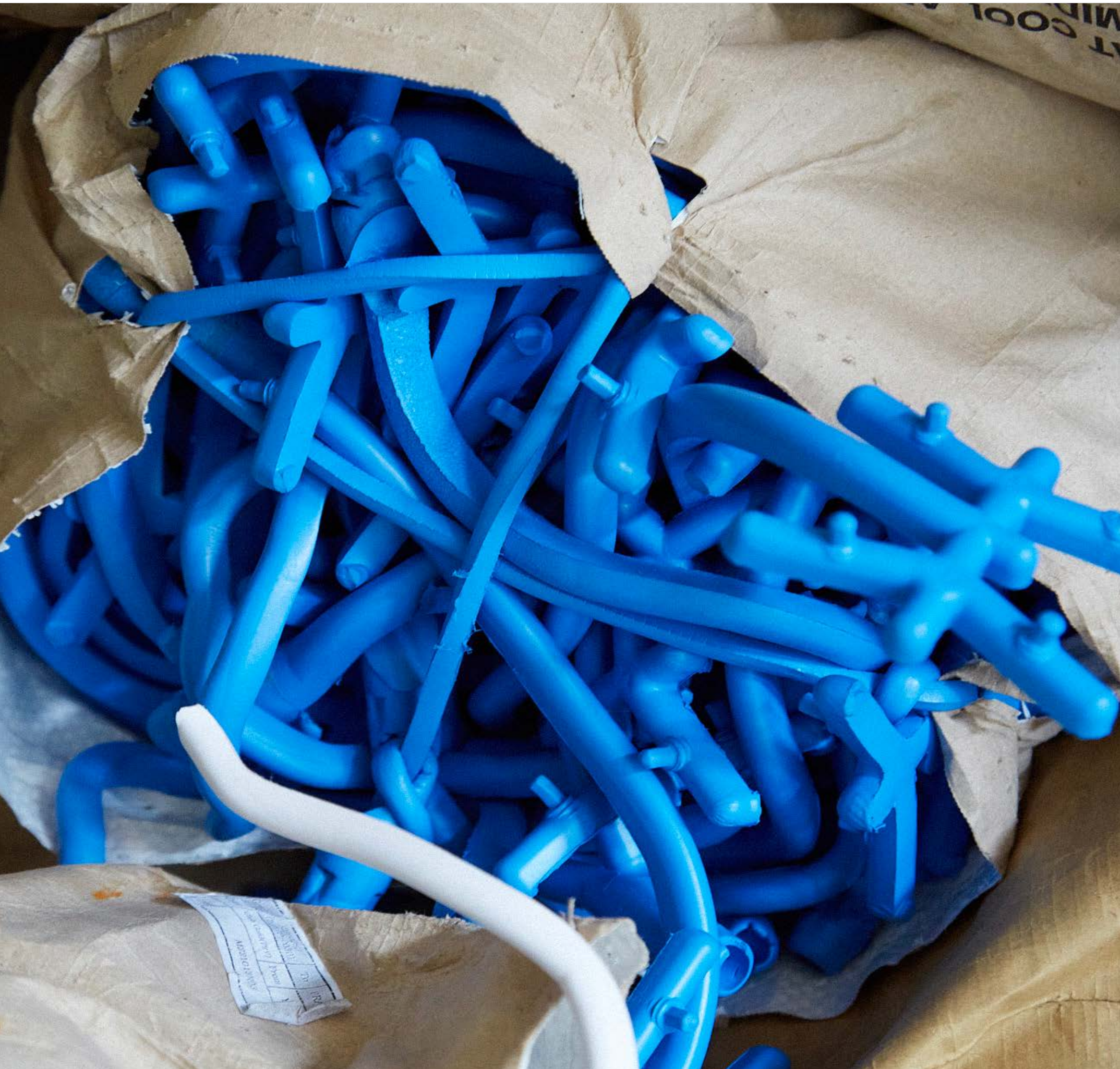
Extra material, called flashing, at the Pratama manufacturing supplier in Indonesia
