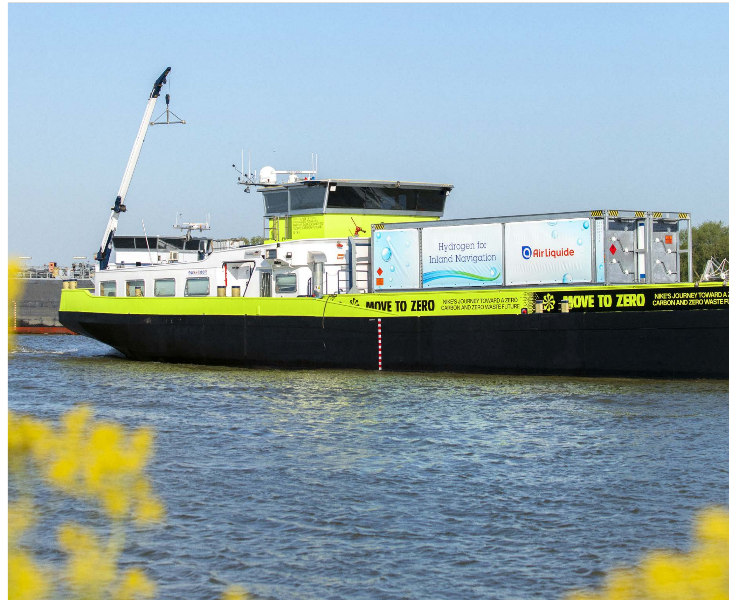
The H 2 Barge 1, a zero-carbon-dioxide-emissions inland vessel
